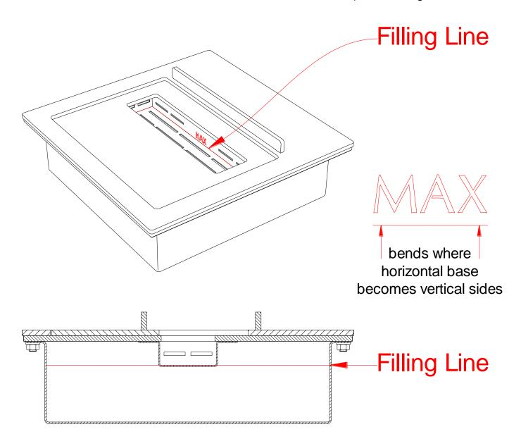
To fill the Combustion Chamber, remove it from the Main Body using the Lifting Handles and pour fuel inside the Vent Opening being careful not to spill. Fill up to the fill line as indicated in red with no more than 1.5L of fuel (3-5 hrs burning time). After filling is done, wipe away any spilled or excess fuel before returning the Combustion Chamber to the Mount Plate opening.
