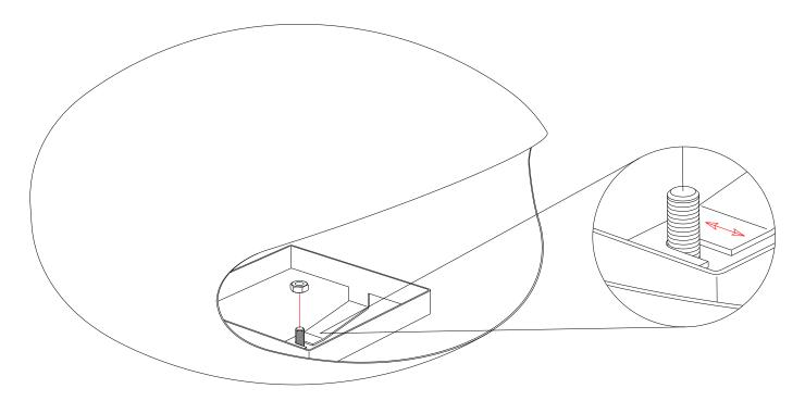
With the Removable Tray Bracket and hex type nut loosely in place, adjust the Removable Tray Bracket backwards or forwards so that the front edge of the Mount Plate (A) sits just below the front bottom lip of the opening in the Main Body (B). Once this adjustment is done, then tighten the hex type nut to secure the Removable Tray Bracket in place.
