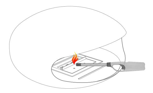
Using a long arm fire lighter and standing at a safe distance from the Combustion Chamber carefully introduce a flame as indicated above to ignite the Combustion Chamber. Always make sure there is a Class B fire extinguisher close at hand when igniting the Combustion Chamber.
