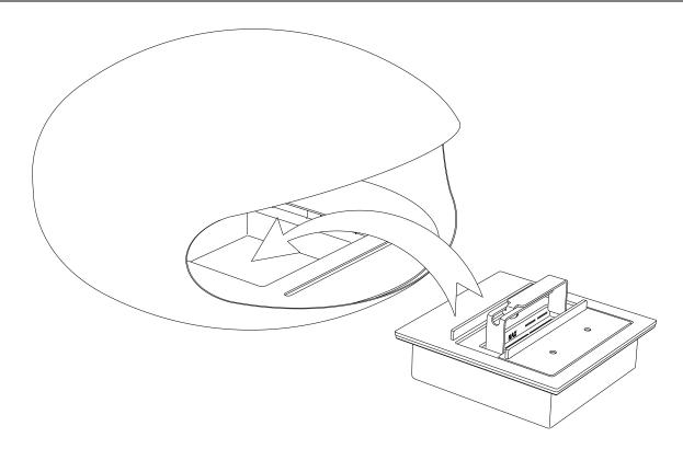
With the Mount Plate in the correct position and secured in place with the hex nut, the Combustion Chamber can now be placed inside and taken off the Mount Plate opening using the Lifting Handles supplied as shown on the previous pages.
