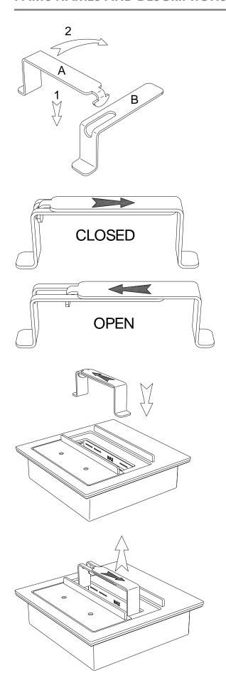
The Lifting Handle is used to take the Combustion Chamber in and out of the Mount Plate inside the Main Body for filling and cleaning. Step 1 is to join Part A and Part B as shown to the left. Once you have placed the tag of Part A into the slot of Part B, then twist it 90 degrees to lock them as one handle.
