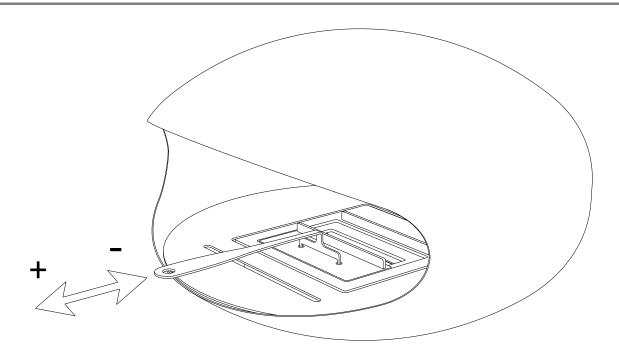
To regulate the flame, insert the tips of the *Sliding Lid Handle* into the holes of the *Sliding Lid* of the *Combustion Chamber* and slide backwards or forwards to regulate the flame size.
