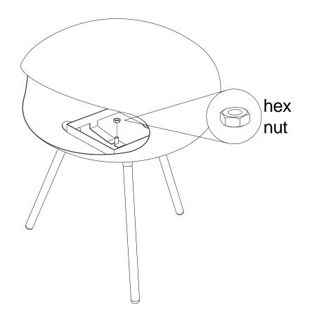
With the Legs securely attached to the Main Body, place the Removable Tray Bracket over the threaded stud at the base of the Main Body, and then tighten in place with the hex nut supplied to be "finger tight". Now follow the adjustment procedures on the following pages before securing with an appropriate tool.
