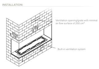
\* The image shows the product with three-side fire view. Other options include two-side view (right/left side and front) and front view.
