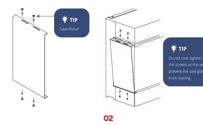
Remove the screws from the blanking plates.
