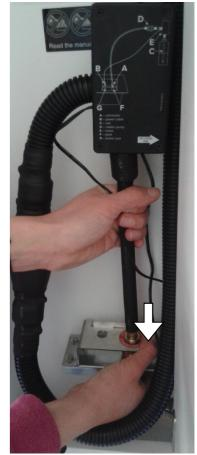
3.2. Place the stiff tube in the external fuel container from which the fuel will be pumped out into the *Lincoln's* fuel tank.
