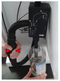
3.4. Connect metal connector of the rigid tube to the matching socket in the cabinet.
