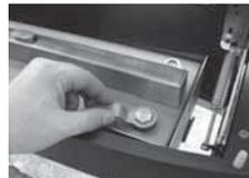
7. Insert the funnel into the filling opening and pour in a maximum of 2.6l of bioethanol.
